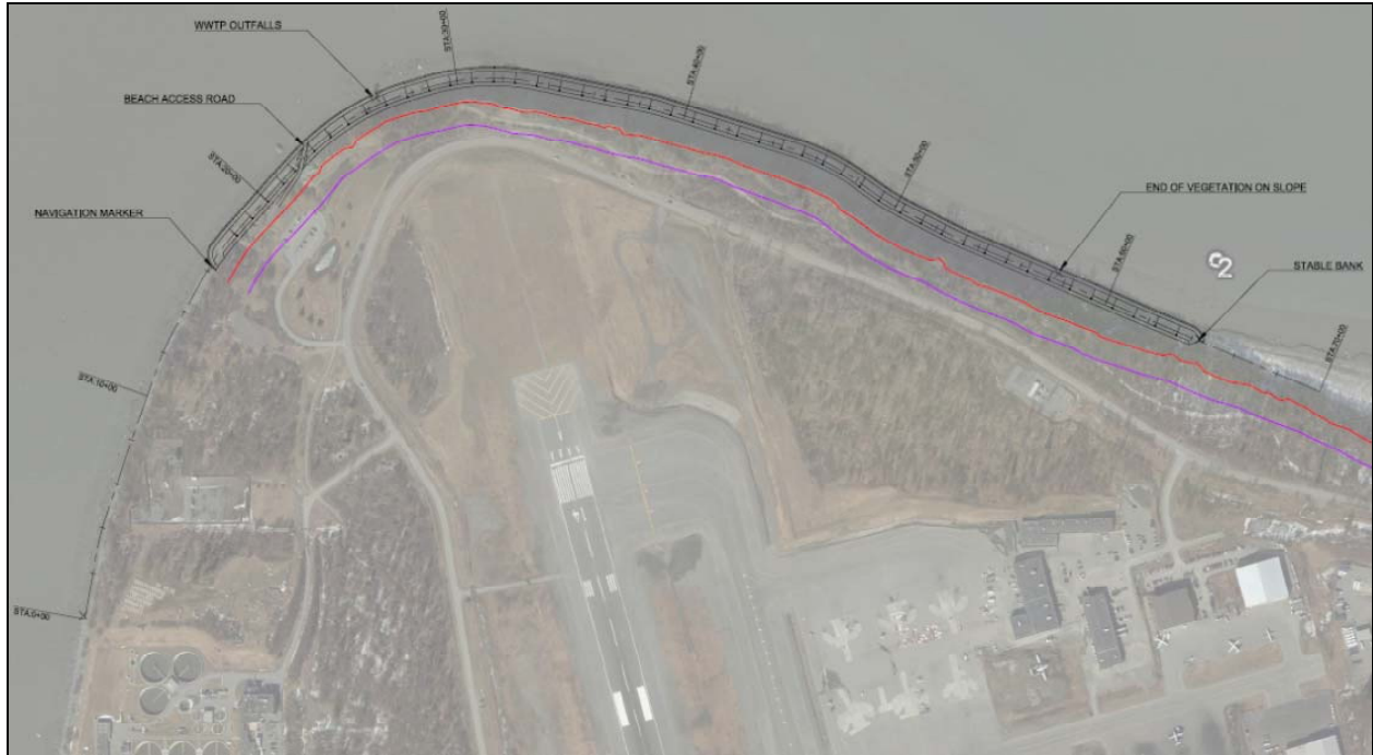
Figure 4: Erosion projection and extent of potential revetment construction. The red line (closest line to water) indicates the top of the bluff in 2015 while the purple line indicates the projected top of bluff in 2065 at an average erosion rate of 2 feet per year.
